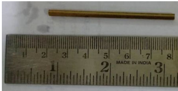
Fig. 22.1 Initial brass tool electrode ( \Phi = 3 mm)
