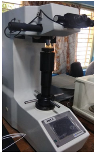
Fig. 15.7 Matsuzawa VMT-X7 for measuring Vickers hardness
