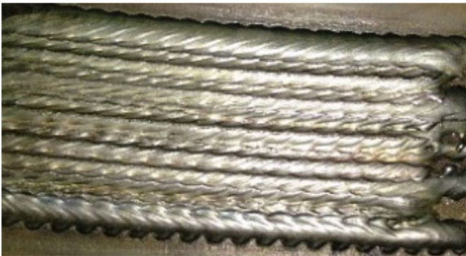
Fig. 49.3 Deposition showing narrow weld bead tracks (lower powder)
