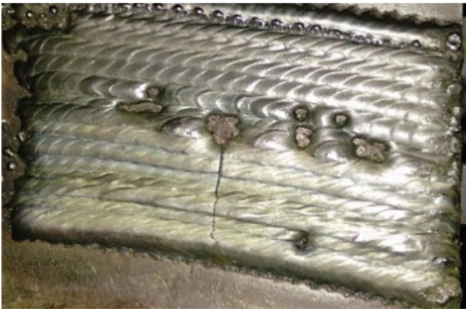
Fig. 49.6 Deposition showing crack overlay (blowholes and gap due to insufficient energy and maximum powder feed rate)
