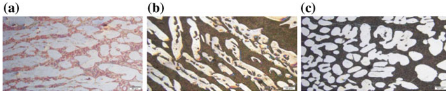
Fig. 62.1 Microstructure of grade 6A quenched from a 850 °C, b 1000 °C, c 1100 °C
