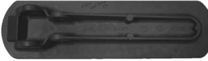
Fig. 47.8 Image of the PDC part after improvement
