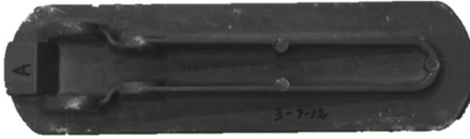
Fig. 47.9 Casting component anodized with high temperature after NSS testing of 242 h
